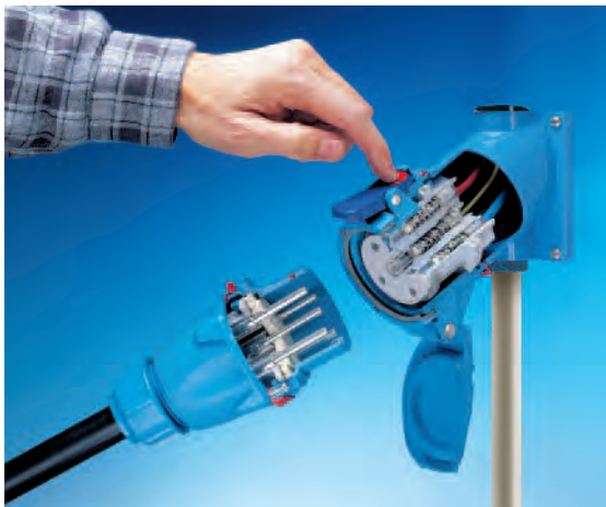
Pressing the pawl/button on the receptacle will safely switch off the DECONTACTOR. The plug can then be withdrawn in complete safety. (Cutaway model shown for illustration purposes)
